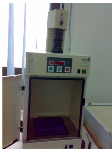
Figure 25: Gel documentation (Gel Doc) with the gel to produce image
