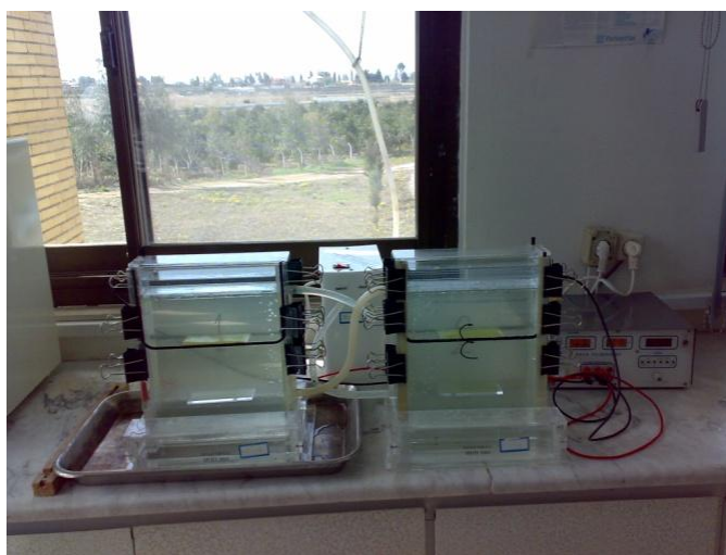
Figure 27: Vertical electrophoresis device and 8% polyacrylamide gel
